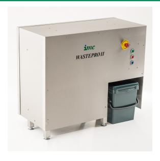
WastePro II is ideal in instances where food waste can no longer be disposed of via mains drainage, either due to technical restrictions or legal regulations. The grey water is dispensed direct to drain whilst the solid waste is captured in a lidded bin for subsequent onward processing. The flexibility of WastePro II provides a cost effective system for commercial and institutional kitchens.
