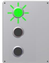
Flashing Green Machine Stopping
