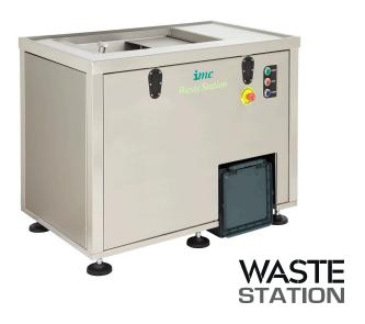
Food waste typically represents around 40% of total commercial catering waste. Of this 40%, approximately 77% is liquid. WasteStation grinds the food waste into fine particles, these particles feed directly into the built-in dewatering system. Through centrifugal action, the WasteStation forces out the excess liquid from the macerated waste.
