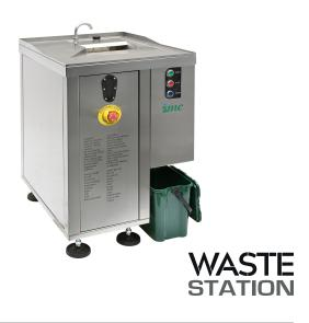
Food waste typically represents around 40% of total commercial catering waste. Of this 40%, approximately 77% is liquid. The WasteStation Compact grinds the food waste into fine particles, these particles feed directly into the built-in dewatering system. Through centrifugal action, the WasteStation forces out the excess liquid from the macerated waste.
