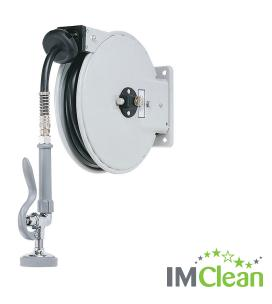
With compact, space-saving design, Reel Kleen 15 hose reels can be mounted on the wall, ceiling or floor. Its 4.5 metre, reinforced rubber hose is ideal for cleaning small to medium-sized kitchen washup areas. It's also retractable, to reduce the risk of tripping. Automatic recoil makes it easy to use and quick to store away. It can be used with water up to 82oC.
